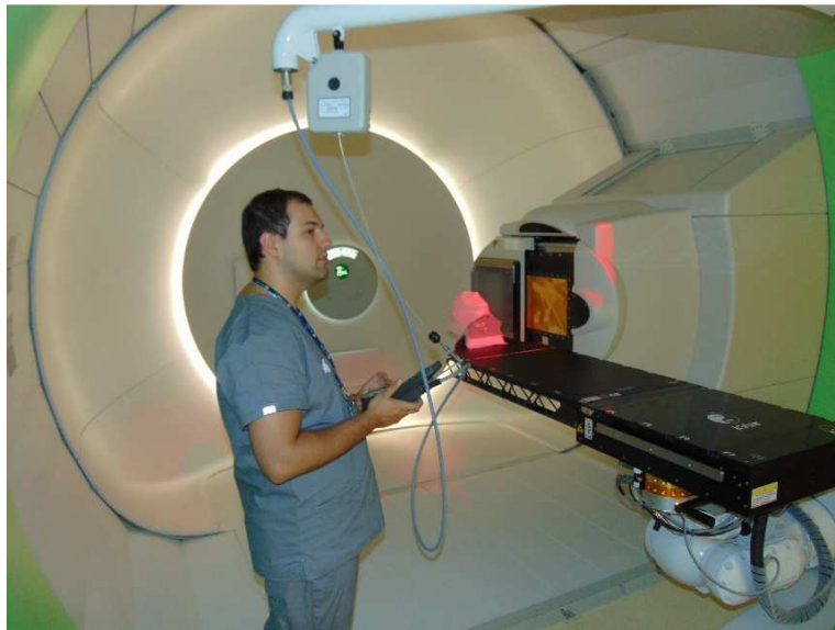
Fig. 4 Positioning of a head phantom at the gantry room at the Cyclotron Centre Bronowice. (copyright: T. Kajdrowicz)
