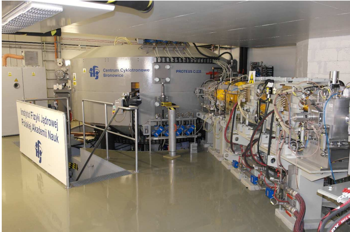
Fig. 3. The Proteus C-235 isochronous cyclotron at the Cyclotron Centre Bronowice, IFJ PAN. (copyright: K. Guguła)
